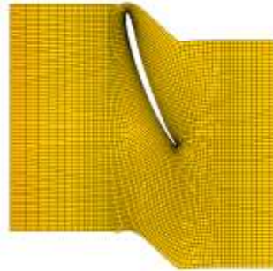
Fig.3.11 Meshing details of Axial pump
